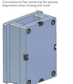
Main guide for rough alignment when closing and assembling
